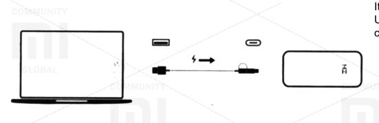
While charging the laptop with USB-C PD or charging a smartphone with Type-C PD, QB820 can charge additional devices simultaneously via two USB-A ports. (For example, feeding power to the mouse and flash drive).
