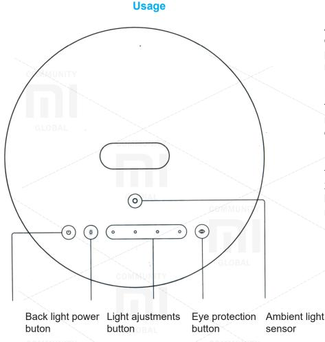
**Power button**: easily click to turn on / off table lamp; press long till indicator flashes, then table lamp reset to factory defaults.
