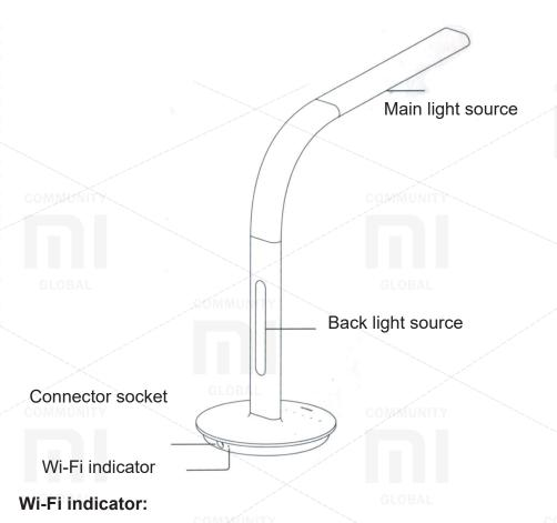
Flashing amber: A standby connection; Slow flashing yellow light: in the process of reconnection; Flashing blue light: in the network connection Long blue light: a successful connection to the router; Fading indicators: Wi-Fi sleep mode.
