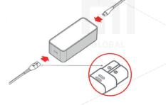
**Cnnecting AC cable** Connect AC cable to power supply.
