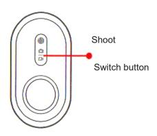
Camera mode: press the shutter button. Video mode: press the shutter button to start/stop shoot video.
