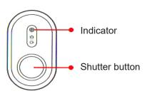
After this, you no longer need to re-connect to the remote control. One click on the shutter button - and you can begin to use the camera. The red light indicates an error in pairing of two devices.
