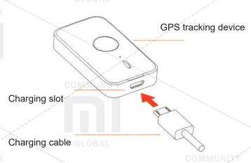
Plug a power adapter into slot, then a flashing green indicator lights up. Charging of the device began. A steady green light indicates a full charge of the device.
