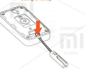
Open a cover of the device, thread a strap through the hole at the bottom of device and fix it.
