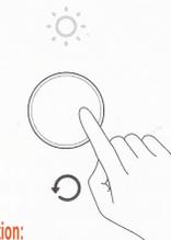
After replacement and the filter and its inclusion, press the button from the back of the air cleaner and hold it within 6 seconds. When some beeps sound, it will specify that replacement of the filter is successfully complete. And the air cleaner starts new counting of term of use of the new air cleaner over again.
