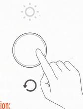
After replacement and the filter and its inclusion, press the button from the back of the air cleaner and hold it within 6 seconds. When some beeps sound, it will specify that replacement of the filter is successfully complete. And the air cleaner starts new counting of term of use of the new air cleaner over again.
