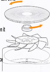
Note: Rotate the impeller clockwise in order to tighten it
