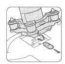
Insert the camera suspension to the slot until it clicks. After setting the PTZ camera installation and dismantling lock will take its original position.
