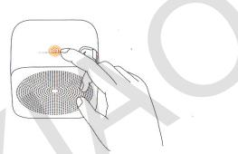
**Play / Pause:** Lightly touch the top of the Mi Internet Radio once to put the radio broadcasting paused. Tap the top bar again to resume playback.
